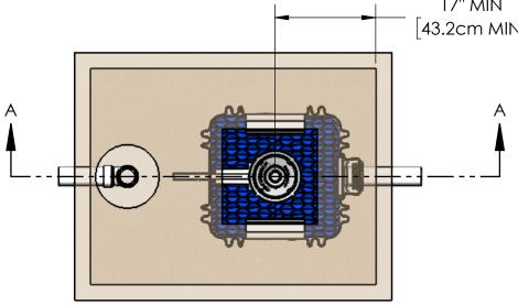
1. AIRLINE PIPING TO FAST® MAY NOT EXCEED 100 FT (30M) TOTAL LENGTH AND HAVE A MAXIMUM OF 4 ELBOWS IN THE PIPING SYSTEM. FOR DISTANCES GREATER THAN 100 FT (30M) CONSULT FACTORY. 2. IF LESS THAN THE SPECIFIED MINIMUMS ARE CONSIDERED NECESSARY,
