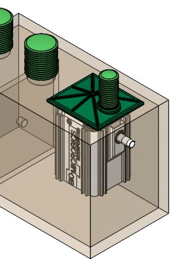
1. AIRLINE PIPING TO FAST® MAY NOT EXCEED 100 FT (30M) TOTAL LENGTH AND HAVE A MAXIMUM OF 4 ELBOWS IN THE PIPING SYSTEM. FOR DISTANCES GREATER THAN 100 FT (30M) CONSULT FACTORY. 2. IF LESS THAN THE SPECIFIED MINIMUMS ARE CONSIDERED NECESSARY, CONSULT FACTORY FOR GUIDANCE.
