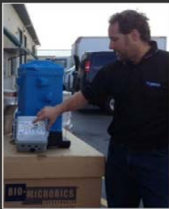
Ray Tebo, of New Excavating Technology, explains how a control panel will tell him exactly how the new BioBarrier membrane bioreactor is working. | Susan DeMar Lafferty/Sun-Times Media
