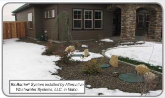
the single family home, the NSF®/ANSI STD 40/245 certified system was installed and has been tested every other month to show the effluent being treated to direct discharge characteristics, i.e. effluent quality of BOD <2 mg/L, TSS <2, Ammonia <1 and reduces Fecal Coliform and E. Coli to less than 10 cfu.
