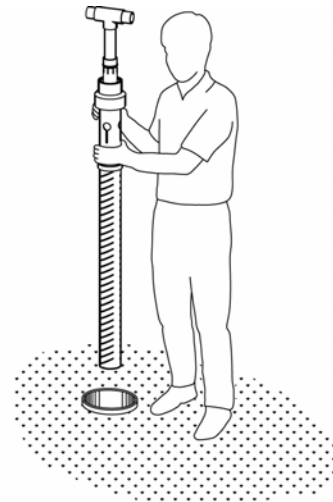
Figure 3: Installation of SaniTEE™
