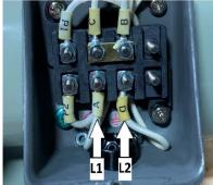
Brass Jumper Connects C & B L1 Connects to A L2 Connects to D
