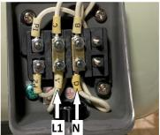
**Brass Jumper 1 Connects A&C Brass Jumper 2 Connects D&B**
